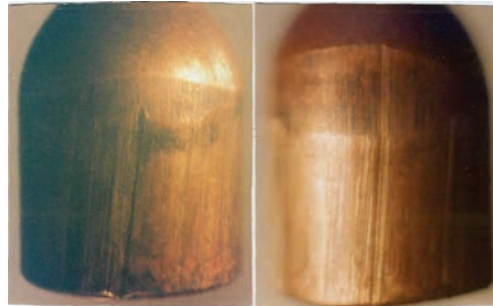
Photo 5. Traces on the surfaces of bullets that were reflected when fired from a craft-made firearm, in which the chamber (photo on the left) and the drum chamber (photo on the right) are misaligned
