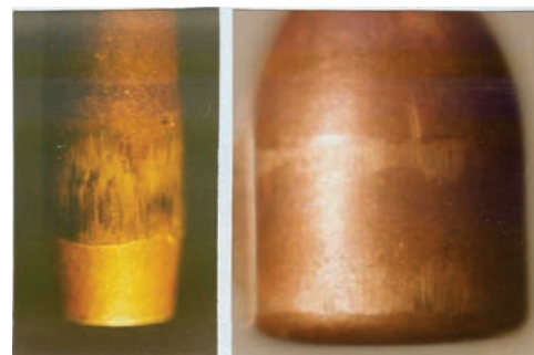
Photo 3. Traces on the surfaces of bullets fired from a smooth-bore craft-made firearm, with the caliber of the barrel channel exceeding +0.5 mm (on the left, bullet from a 5.45x39 cartridge, on the right, from a 9x18 cartridge)
