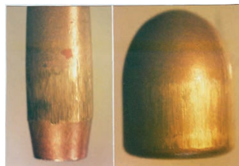
Photo 2. Traces on the surfaces of bullets fired from a smooth-bore craft-made firearm, in which the caliber of the barrel channel is 0.1 mm larger (left – bullet from a 5.45x39 mm cartridge, on the right – 9x18 mm)
